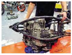
25: With all the peripherals removed I can now remove the engine bolts and lift the frame off the engine. It's a bit of a wiggle to clear it, but at this stage I'm not worried about scratching any paintwork. The engine will stay on the bench for stripping down, and I now have a big pile of dirty, greasy parts to clean up and check over before sending them out for re-finishing. And then, I'll have to come up with a plan for the bent frame.
