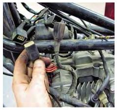
13: Time to unplug the harness and unbolt the coils, and store them all away in the Big Box of Electrical Stuff for sorting out later on. A quick examination shows the harness to be in pretty sound nick – there's no obvious signs of bits of bodged wiring repairs that we see so often. Even the block connectors look pretty good, but it will all be cleaned up and checked over before I assume any of it is fit to reuse.
