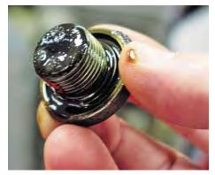
O3: While I'm working on the rest of the bike I'll remove the oil drain plugs, so any old lubricant in there can drain safely away. Encouragingly, the sump drain bolt unscrews fairly easily – these can be tight on older Z1s and I've even heard of someone cracking a sump while trying to unscrew one. The drain bolt is magnetic and has a fair bit of metallic sludge stuck to it. Possibly evidence of missed oil changes, which somehow doesn't surprise me. Hopefully the engine internals aren't too bad.
