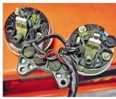
17: The clock assembly comes away from the top yoke after removing two bolts. Again, all the rubber mountings are perished so everything's wobblier than it should be, but that's all easily fixable. The tacho head, though, is quite obviously damaged so I'll be going shopping for a second-hand item to replace it. This lot will dismantle further, but again I'm taking lots of pictures of the wiring to help me put it back together correctly when I rebuild the bike later.
