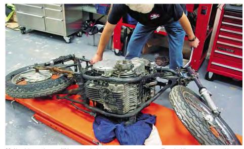
22: Next job – engine out. With rags on the bench to prevent any more scuffing, the bike now goes over sideways. I'm taking the engine out as one lump, and will treat it as a project in itself. With all the weight on the engine I can now remove the wheels and suspension, leaving me with the fairly easy task of lifting the main frame loop off the engine on the bench. At this stage it's also easy to get at the main engine mounting bolts and loosen them all off.
