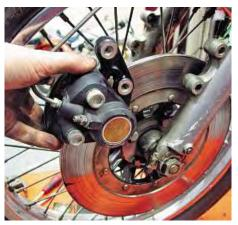
21: The caliper is correct for the Z1 at least, and it looks to be in fairly good nick, apart from a little light scuffing. I have no idea if it actually works, but for now I'll unbolt it and store it for a full strip down later. The marks on the fork leg could be accident damaged, or could simply have been caused by the bike rattling around in a transatlantic container. The sticker on the fork leg is an authentic touch of the bike's US heritage.
