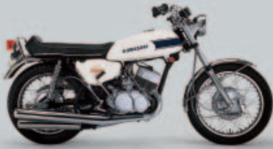
1969 H1 | KH500-A 2-stroke Air-cooled In-Line Triple Piston valves 498 cm 3
