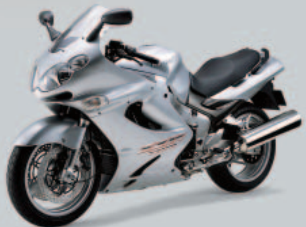
2002 ZZ-R 1200 | ZX1200-C 4-stroke Liquid-cooled In-Line Four DOHC, 16 valves 1,164 cm 3
