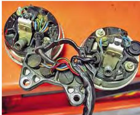
17: The clock assembly comes away from the top yoke after removing two bolts. Again, all the rubber mountings are perished so everything's wobblier than it should be, but that's all easily fixable. The tachometer head, though, is quite obviously damaged so I'll be going shopping for a second-hand item to replace it. This lot will dismantle further, but again I'm taking lots of pictures of the wiring to help me put it back together correctly when I rebuild the bike later.
