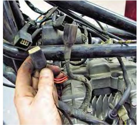
13: Time to unplug the harness and unbolt the coils, and store them all away in the Big Box of Electrical Stuff for sorting out later on. A quick examination shows the harness to be in pretty sound nick – there's no obvious signs of bits of bodged wiring repairs that we see so often. Even the block connectors look pretty good, but it will all be cleaned up and checked over before I assume any of it is fit to reuse.
