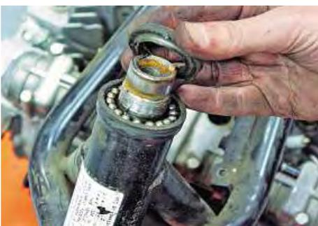
24: Now, at last, the top yoke can be removed. The head bearings were a little notchy but I intend to fit taper rollers as part of the rebuild. While I want to (hopefully one day) experience the undiluted Z1A riding experience I fully intend to take advantage of modern bearing technology at both the steering head and swingarm pivot. It's hard to imagine a time when cup and cone bearings from a bicycle were considered adequate for the most powerful production motorcycle in the showrooms.
