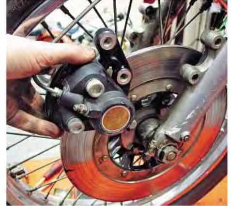
21: The caliper is correct for the Z1 at least, and it looks to be in fairly good nick, apart from a little light scuffing. I have no idea if it actually works, but for now I'll unbolt it and store it for a full strip down later. The marks on the fork leg could be accident damaged, or could simply have been caused by the bike rattling around in a transatlantic container. The sticker on the fork leg is an authentic touch of the bike's US heritage.
