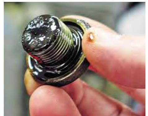
03: While I'm working on the rest of the bike I'll remove the oil drain plugs, so any old lubricant in there can drain safely away. Encouragingly, the sump drain bolt unscrews fairly easily – these can be tight on older Z1s and I've even heard of someone cracking a sump while trying to unscrew one. The drain bolt is magnetic and has a fair bit of metallic sludge stuck to it. Possibly evidence of missed oil changes, which somehow doesn't surprise me. Hopefully the engine internals aren't too bad.
