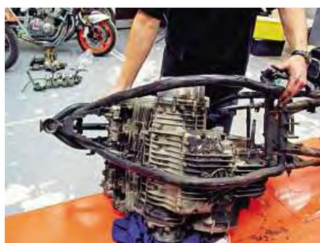
25: With all the peripherals removed I can now remove the engine bolts and lift the frame off the engine. It's a bit of a wiggle to clear it, but at this stage I'm not worried about scratching any paintwork. The engine will stay on the bench for stripping down, and I now have a big pile of dirty, greasy parts to clean up and check over before sending them out for re-finishing. And then, I'll have to come up with a plan for the bent frame.
