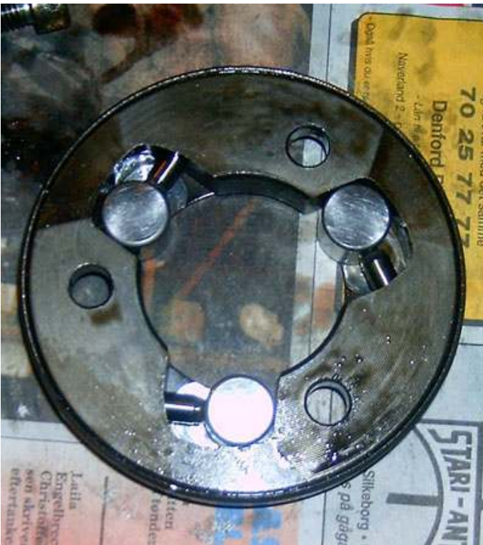
pic 5 – starter clutch disassembled, top flipped over
