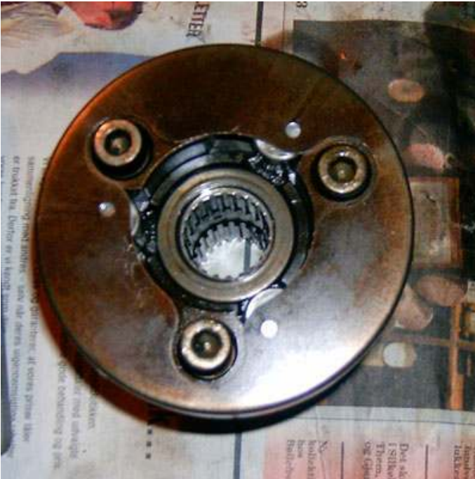
pic 4 – starter clutch w/starter sprocket removed
